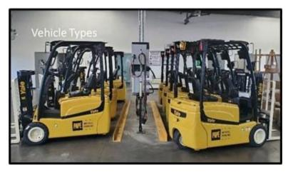
can be moved on these vehicles. There are subtypes and mature vehicles. Electric drive forklifts have lower rates of efficiency. DHE's goal is to substitute the petroleum fueled vehicles with lithium ion and zero maintenance batteries.
