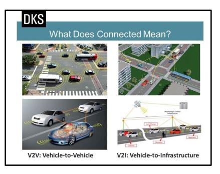
connected components talking to infrastructure in vehicles, then this could become one more sensor input. "Where the vehicle uses not only localized sensors to see what is going on around it, but it is actually talking to other vehicles. And when it is talking to other vehicles saying, 'I am here, here is my speed and heading and I have my right turn signal on and I might be coming your way," said Pearmine.
