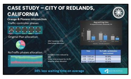
After the smart traffic signal was installed, the system can calculate the demand from all of the users in real time. From there, intelligent decisions are made on how to allocate the right amount of green time most efficiently. According to Lindsted, there was a 60% reduction in delay, which was equivalent to adding 60% street capacity without having to build any real infrastructure.
