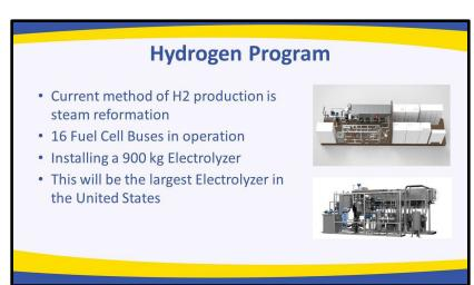
electrolyzer in the United States, with the goal of producing 900 kilograms using solar energy. An electrolyzer is a device that uses an anode and cathode to separate water into hydrogen and oxygen.
